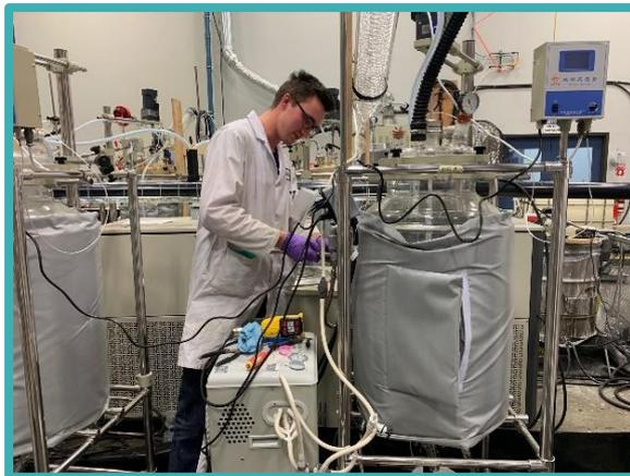
Second stage boric acid crystalliser at Ioneer's pilot plant in Vancouver.
