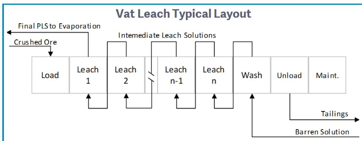
Vat leach offers a high degree of control over leach kinetics – resulting in a reliable, repeatable and robust leach process. Vat leaching also achieves relatively high concentrations of lithium and boron into PLS. The higher concentration in the vat leach PLS means less evaporation and subsequently, lower energy consumption. For further information on the advantages of vat leaching Rhyolite Ridge mineralisation, see the Global Geoscience announcement dated 23 May 2018.
